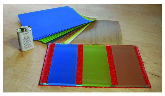
Our recommendation is to use the 40, 30 and 5 micron films for day-to-day sharpening of chisels and plane irons, a couple of light pull strokes on each should be all that is necessary for a well prepared blade.
