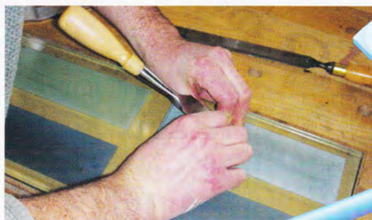
Freehand honing on the bevel
